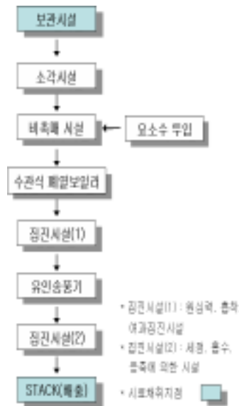
Fig. 5. Schematic of waste incinerating plant
