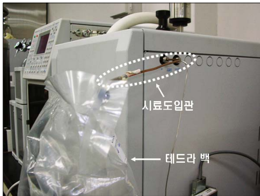
Fig. 4. Before Tedlar bag and Line heating on SPT-GC/NPD
