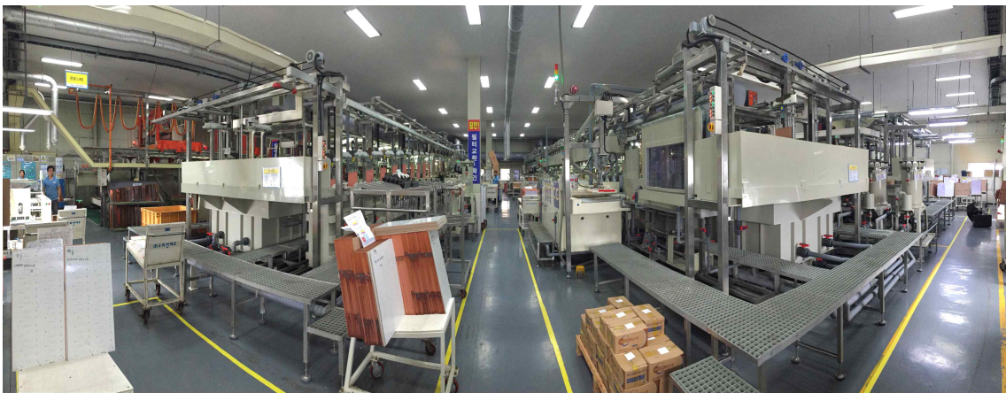
Fig. 34. Panel plating process of Printed Circuit Board Factory.
