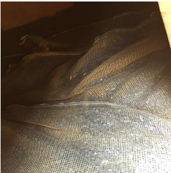
Fig. 20. Pigment attached to on activated Carbon
