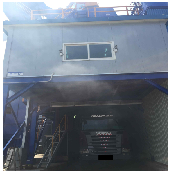
Fig. 12. Process of loading an ascon in a vehicle.
