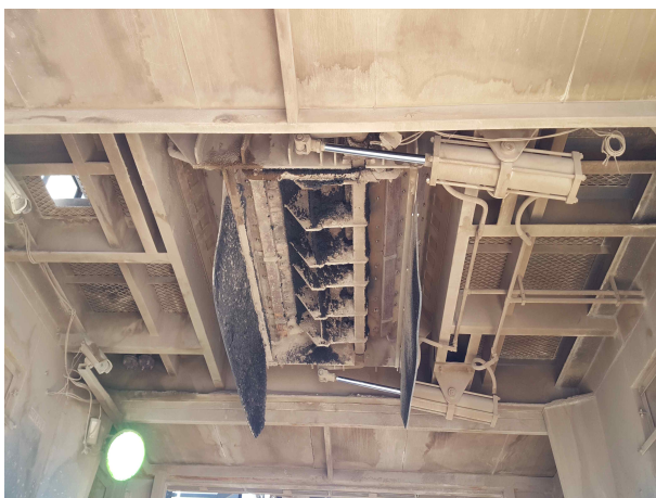
Fig. 13. The inside of the ascon hopper and the air curtain.
