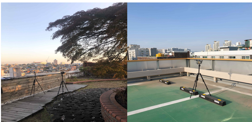
Fig. 4. Measurement of rooftop (Left : Application of green roofs, GR, Right : Non-Application of green roofs, NGR)
