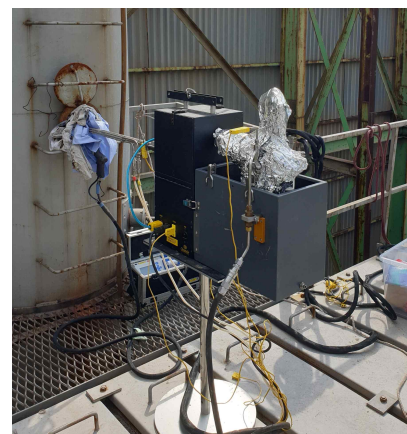
Fig. 6. Flow-chart(Left) and Actual place(Right) of PAHs sampling system from stack
