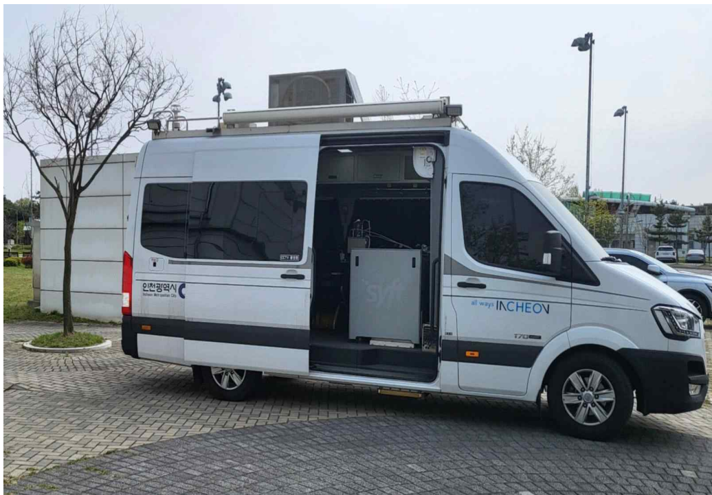
Figure 3. Real-time Odor Analysis Vehicle for the Monitoring of Odor used in this study : (a) Outside View, (b) Selected Ion Flow Tube-Mass Spectrometry
