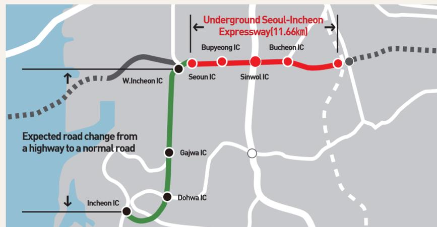
Incheon Metropolitan City is planning to place a part of the Gyeongin Expressway between West Incheon Interchange and Sinwol Interchange (11.66) underground and to turn the overhead ground area into a regular road and park.
